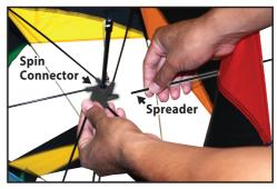
2 Insert Each Spreader into Spin Connector.
