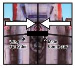
**4.** Insert Wing Spreaders, left and right, into the Main Connector.
