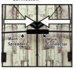
**3.** Insert Main Spreaders, left and right, into the Main Connector.
