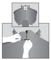
2. Insert Spreader (without cap) into Spine Connector (left and right).
