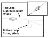
4. Attach the QuikClip® to the Bridle on front of kite.
